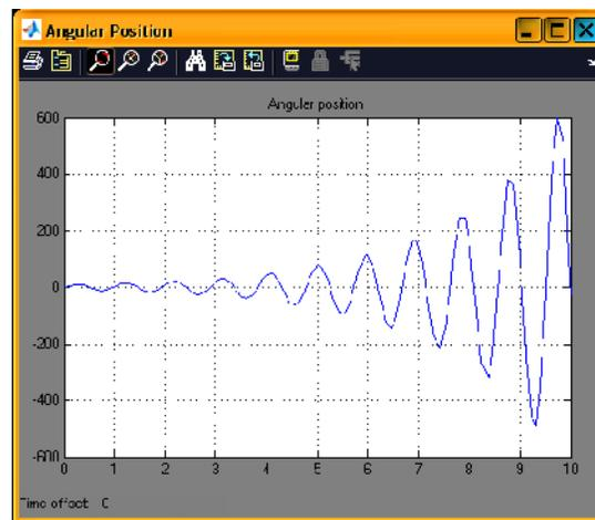
Fig. 11. Angular position for a 0.05pu change in mechanical input with K5 negative.
